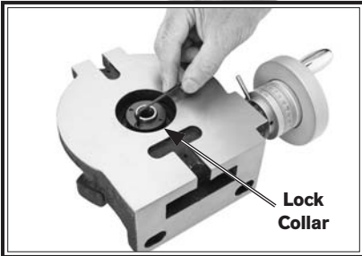
Figure 16. Loosening the spindle lock collar cap screw.
